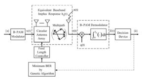
Figure 1. Block diagram of the simulated system
