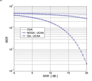
Figure 4. BER V.S. SNR over Scenario for three kinds of transmitter
